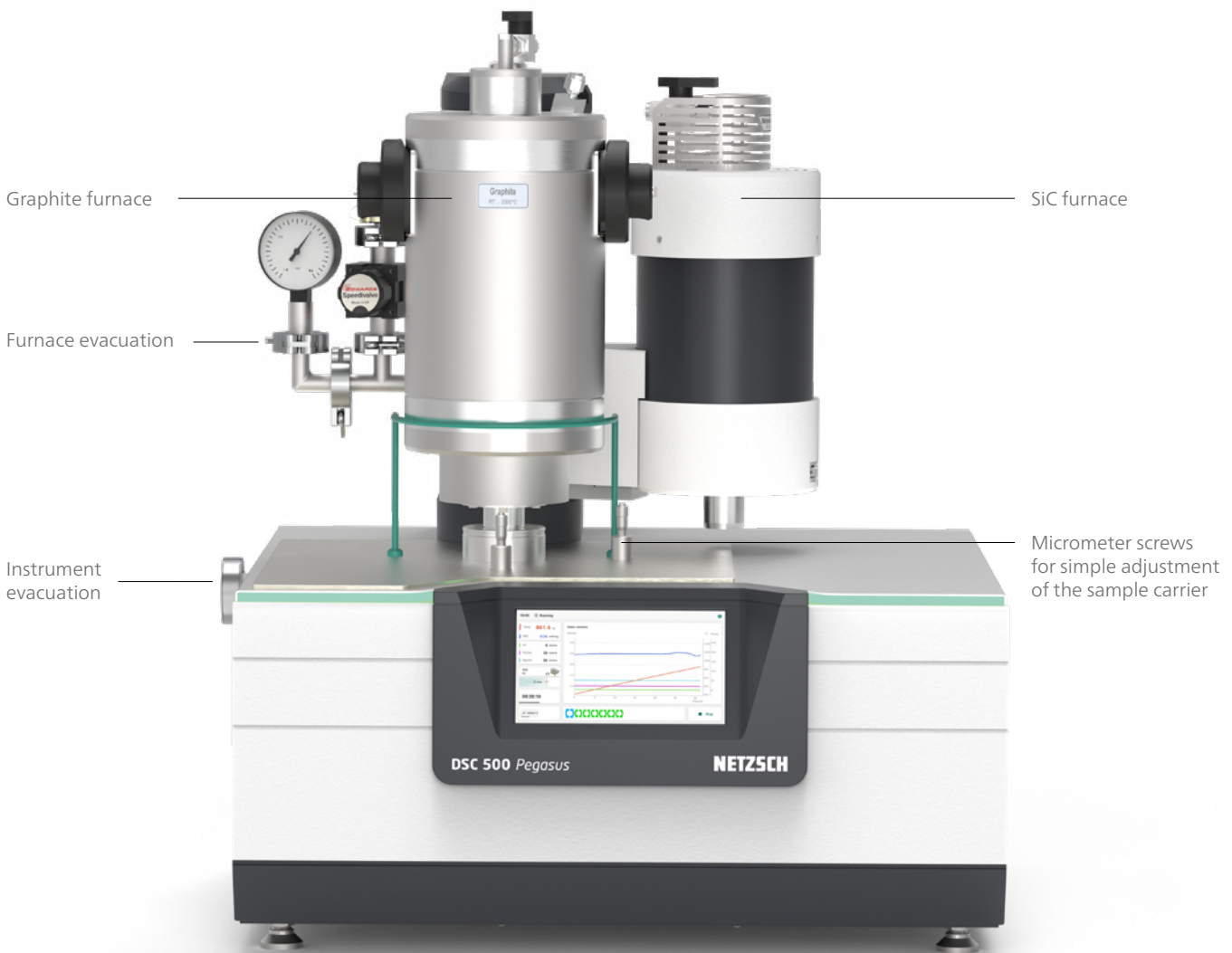
DSC 500 Pegasus ® with graphite and SiC furnace
