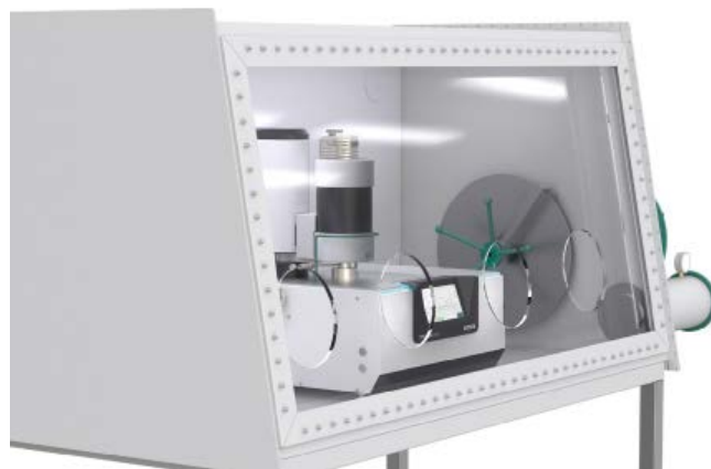
1 A NETZSCH STA inside a glovebox
