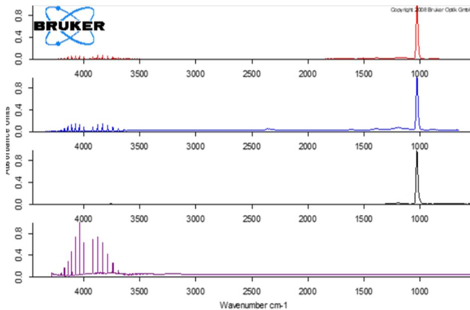
4 Extracted spectra at 460°C (red) and 570°C (blue) compared to the library spectra of SiF<sub>4</sub> (black) and HF (purple).
