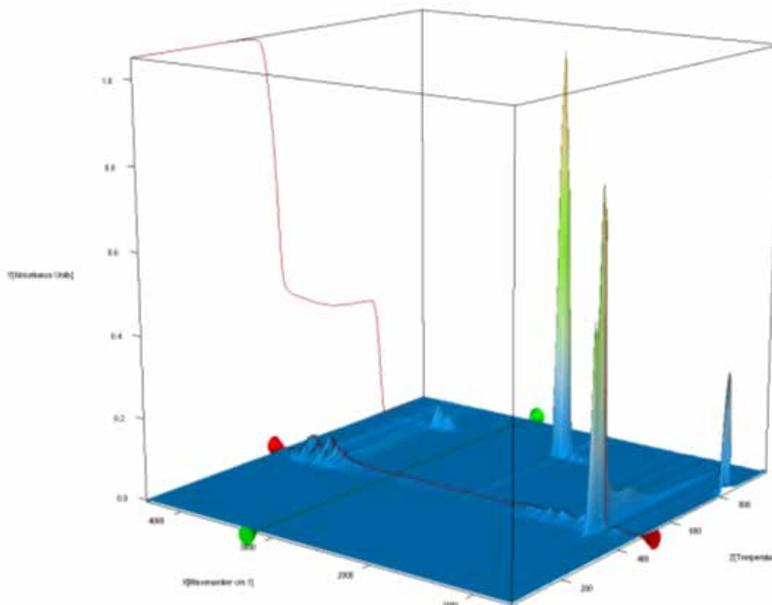
3 3D plot of all detected IR spectra of pure PVDF, TGA curve plotted in red at the back of the cube
