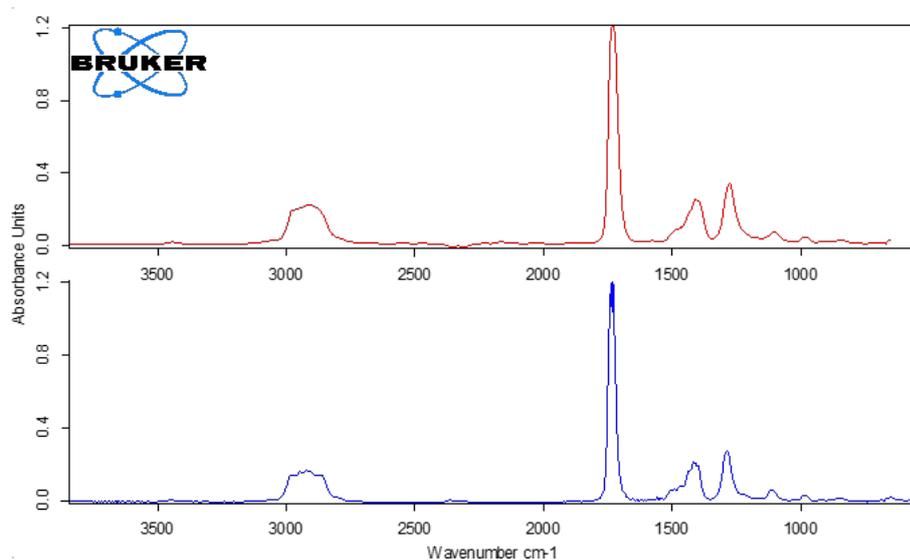
6 Extracted spectra of PVDF in NMP (red) at 155°C compared to the library spectra of NMP (blue).
