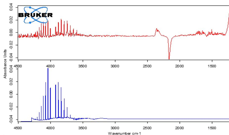
7 Extracted spectra at 432°C (red) of PVDF in NMP compared to the library spectrum of HF (blue).
