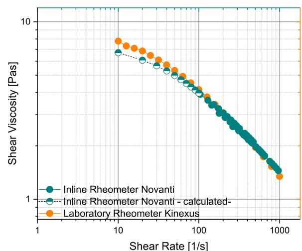
Comparison of viscosity measurements in-line (green) and off-line (orange) of slurries during the production of LFP cathodes
