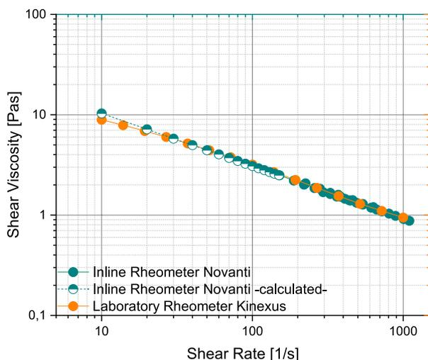
Comparison of viscosity measurements in-line (green) and off-line (orange) of slurries during the production of anodes
