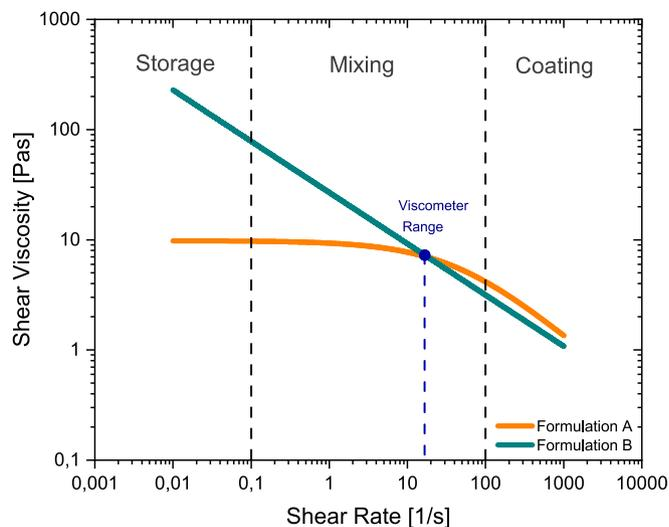
**Viscosity profiles:** Slurries exhibiting similar flow behavior at high shear rates (processing conditions) can still differ significantly in their low-shear (storage) properties.
