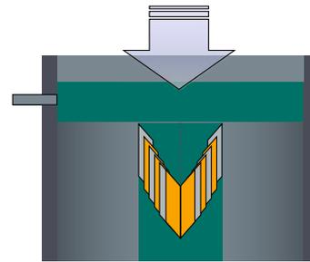
Scheme of the slit die including slurry flowing through the die (yellow)
