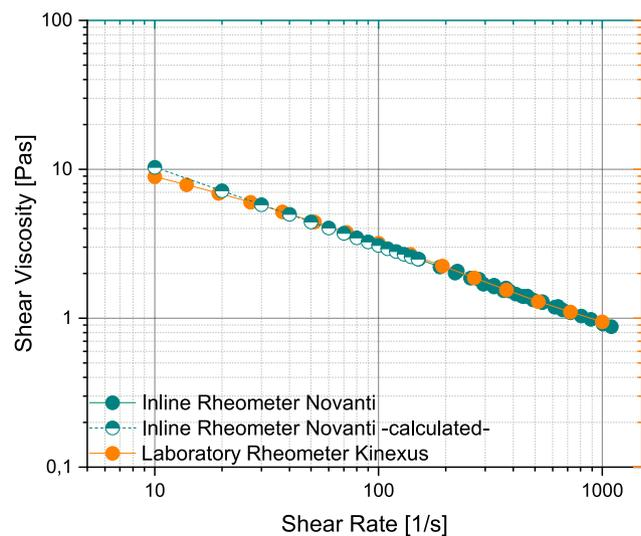
Data comparison between in-line and lab measurements
