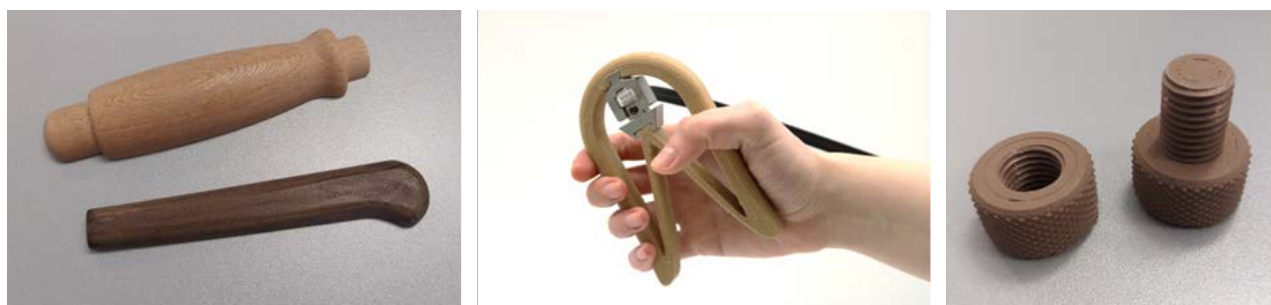
1 Example applications for wood-filled filaments in knife and tool handles (left), demonstrator of crimping pliers based on compliant mechanisms (center), and a printed screw with nut made of bronze-filled filament (right).
