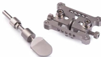
Sample holder set for shearing with flat surfaces
