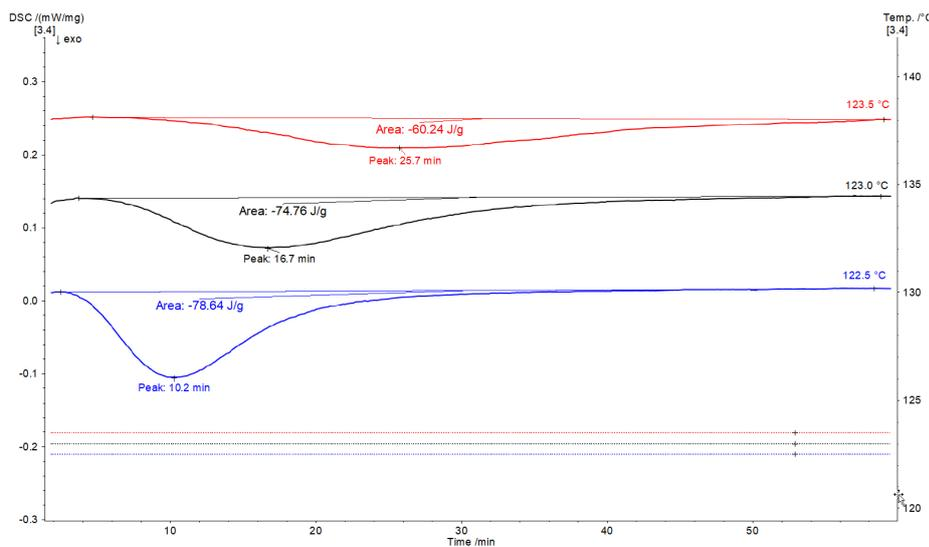
2 Isothermal crystallization of HDPE at 3 different temperatures
