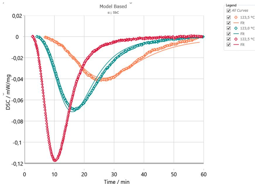
**3** Comparison of the measurement curves (symbols) with the calculated curves (continuous lines).
