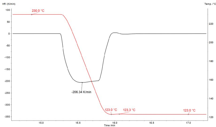
1 Temperature profile of the cooling run to 123°C
