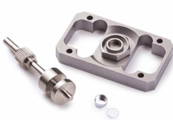
Frame with sample insert, pushrod and sapphire disc for compression measurements on pasty samples. The use of aluminum pans (NGB810405) prevents sample holder contamination.
