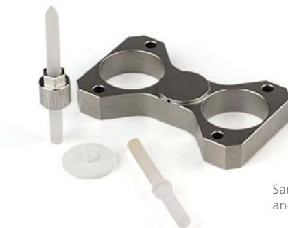
Sample holder set for measurements on insulation foam and for TMA measurements (DMA2420CA52.030-00)
