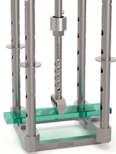
Stiff samples such as fiber-reinforced or highly filled thermoplastics, metals or ceramics can be measured in three-point bending. A special advantage of this geometry is that no clamping effects will influence the results.
