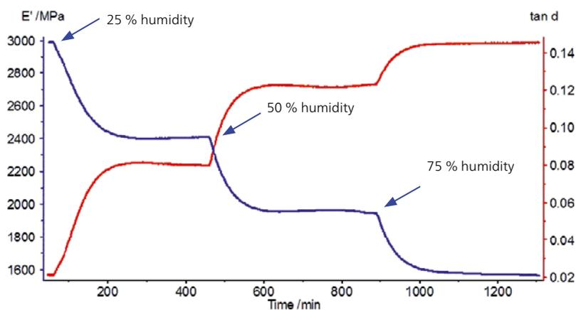
DMA measurement with humidity generator
