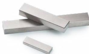
Steel Bars for System Stiffness Calibration
