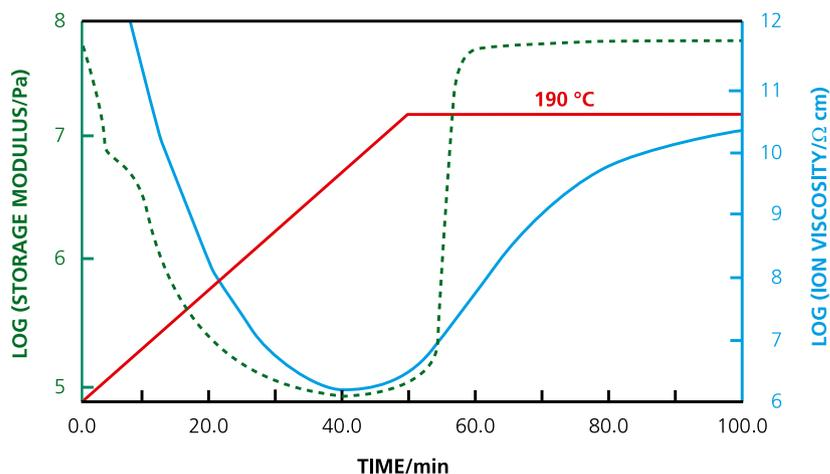
Curing of an epoxy resin
