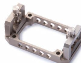
The 17-mm and 20-mm frames for single cantilever with reinforced clamps are used for measurements on very stiff samples.
