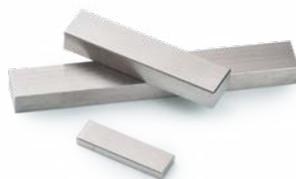
Steel bars for system stiffness calibration
