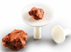
Al 2 O 3 slip-on plates ( \varnothing 17 mm, 10 mm)
