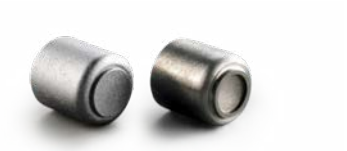
Tungsten crucible (right) and graphite crucible (left)
