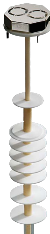
DSC sample carrier type S (Pt-Pt10%Rh)
