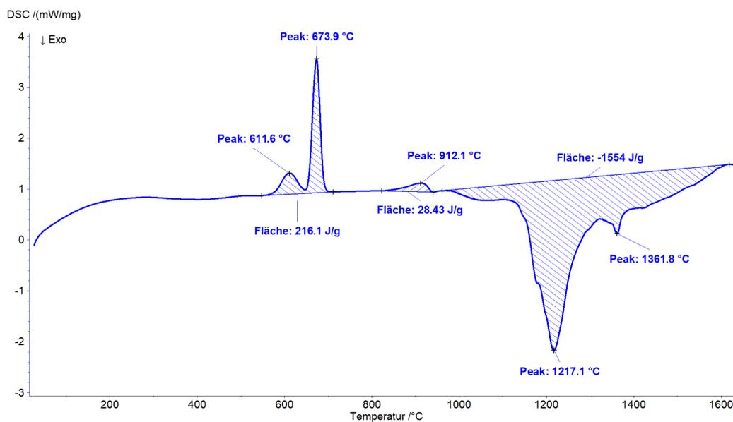
1 DSC curve of the sample mixture of manganese ore and aluminum granulate (at a ratio of 1:1) at a heating rate of 20 K/min.
