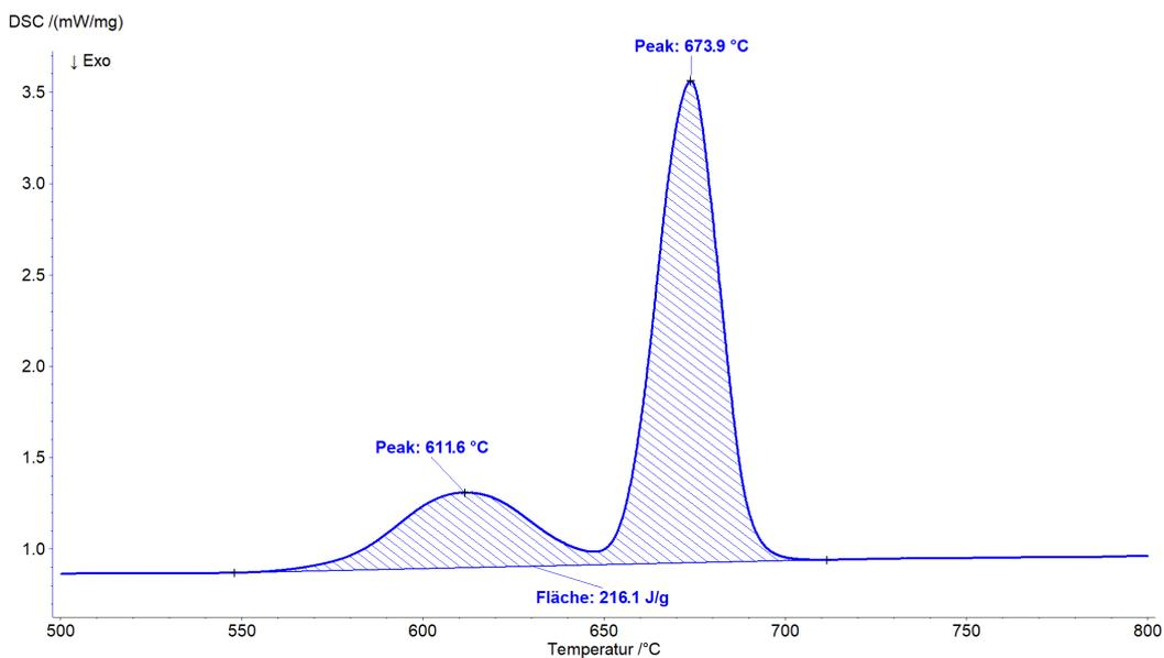
2 Section of the DSC curve in the temperature range from 500°C to 800°C.
