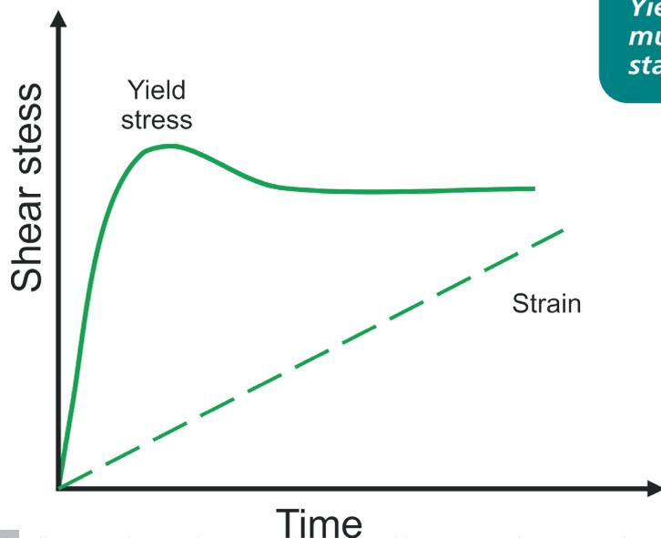
*Yield stress is defined as the stress that must be applied to the sample before it starts to flow.*
