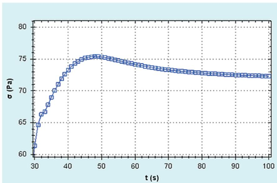
2 Stress ( $\sigma$ ) versus time curve for a body lotion sample run at a constant shear rate of  $0.01 \text{ s}^{-1}$
