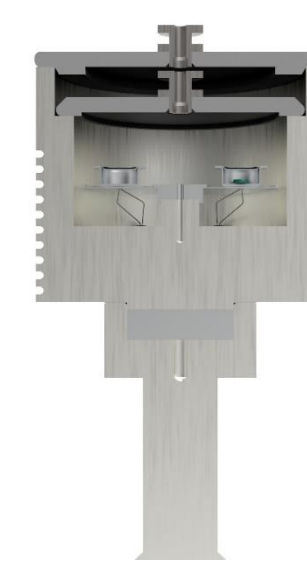
Fig.4 Schematic of the DSC sample holder.
