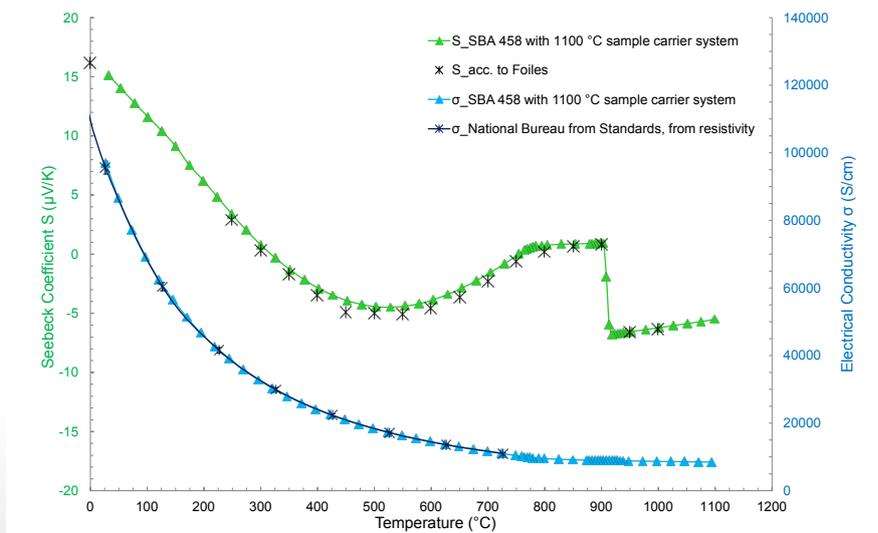
5 Measurement of the Seebeck coefficient and the electrical conductivity of pure iron with the SBA 458 in comparison with literature – Sources [2] and [4]
