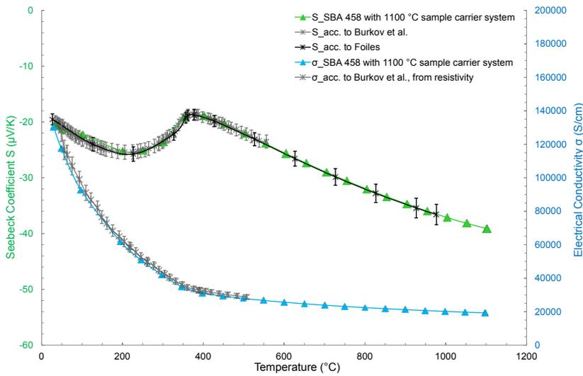
**2** Measurement of the Seebeck coefficient and the electrical conductivity of nickel with the SBA 458 in comparison with literature – Sources [1] and [2]
