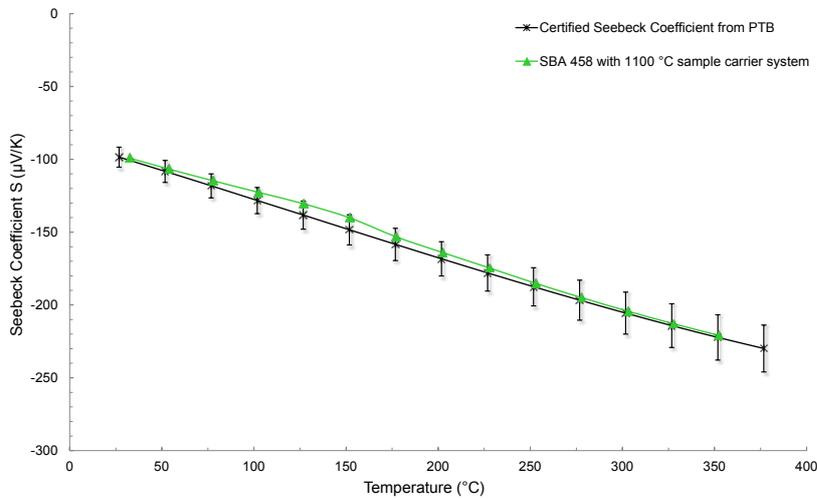
4 Measurement of the Seebeck coefficient of the certified lead telluride, PbTe, with the SBA 458 in comparison with literature – Sources [1] und [2]
