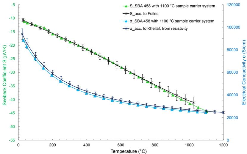
**3** Measurement of the Seebeck coefficient and the electrical conductivity of palladium with the SBA 458 in comparison with literature – Sources [2] and [3]
