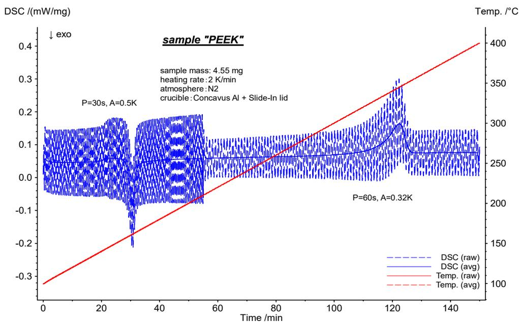
2 Raw DSC signals of the TM-DSC measurement on the "PEEK" sample
