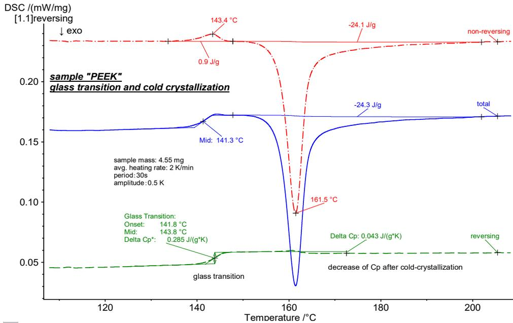
3 TM-DSC results for the glass transition and cold crystallization for the "PEEK" sample.
