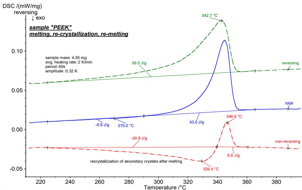
4 TM-DSC results for melting, re-crystallization and re-melting for the "PEEK" sample.
