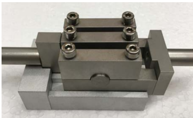
3 Fully assembled sample holder with steel cylinder, inserted using the alignment tool.
