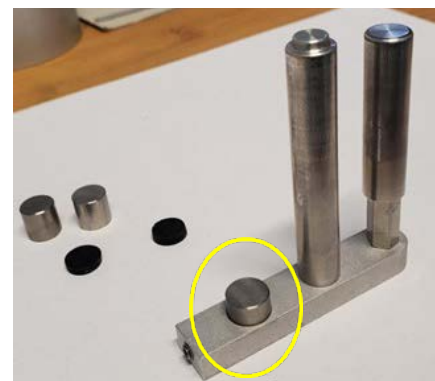
2 Photo of the insertion tool kit with the steel cylinder placed in the depression and tightened with the grub screw.
