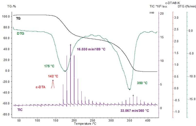
3 TGA results (black), DTA results (green), c-DTA<sup>®</sup> signal (red) and total ion chromatogram of the ASA measurements (purple)
