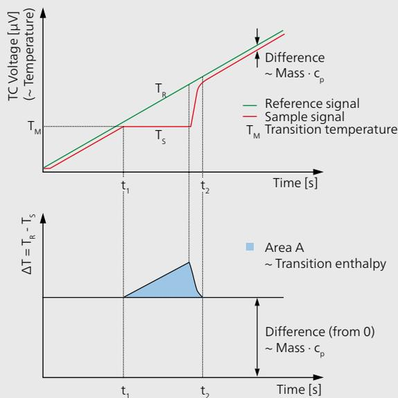
Signal generation in a heat flux DSC
