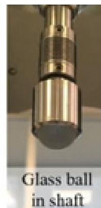
1 Schematic of the measuring geometry and the tribosystem (left), sample holder with cocoa mass sample (middle), and upper geometry with glass ball (right)
