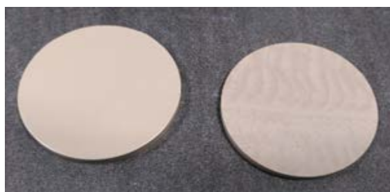
2 Pure PPS, 5 mm (left) and 4 mm (right), with inhomogeneity (pores in the light parts).
