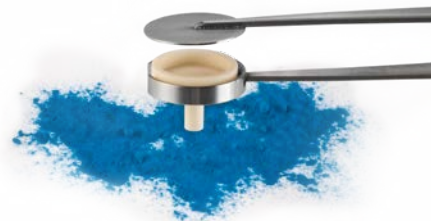
Al 2 O 3 crucible for glove box applications
