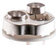
DSC sensor in round design with Pt crucibles
